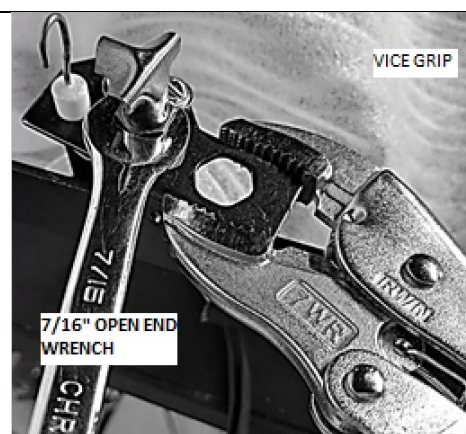
Figure 4-15 Pinch Pilot Base with Vice Grips
